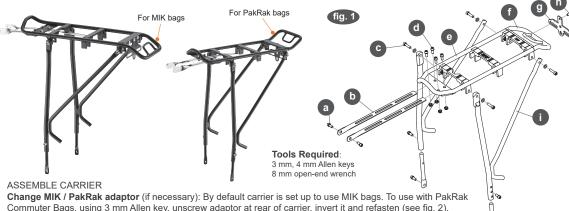
Commuter Bags, using 3 mm Allen key, unscrew adaptor at rear of carrier, invert it and refasten (see fig. 2). **Assemble legs:** Measure distance from lower carrier bolt holes (on dropouts) on your bike. Choose Width A or B according to whichever more closely matches your measurement (see fig. 3).
